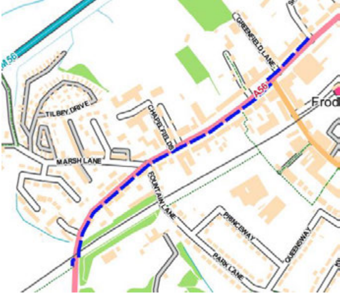
Above: The long-term option of connecting Ship St to FP33 via the south side of Main St. Between Church St and Fountain's Lane segregated infrastructure would provide a long-term solution but require re-alignment of parking spaces to Coward's butchers, then the use of the existing carriageway to Fountain's Lane. The footway to the Castle Park entrance is more suitable for Shared Use than the northern side. (photo)
